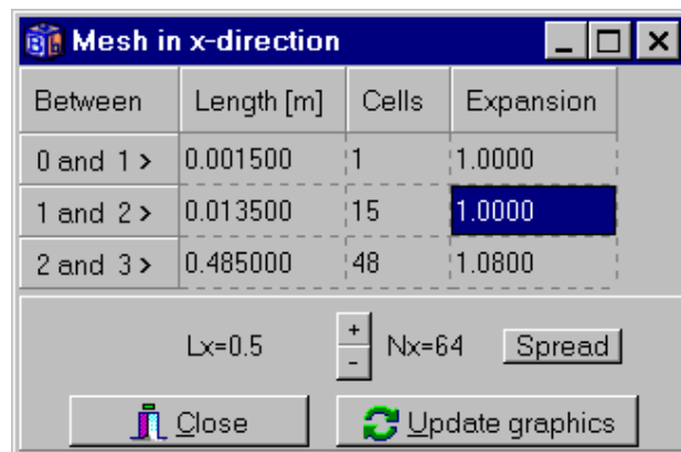
Figure 8.43: The numerical mesh is changed to an expansive mesh in the x -direction.
