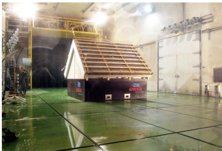
Picture 2: Test house during rain-test
