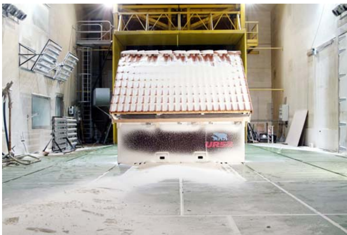
Picture 7: Test house after snow-test
