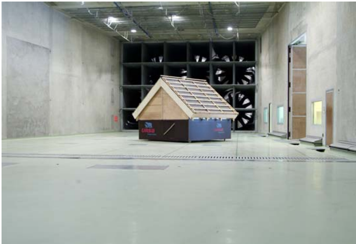
Picture 1: Test house in the wind tunnel
