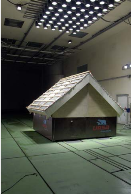
Picture 3: Test house during summer-test
