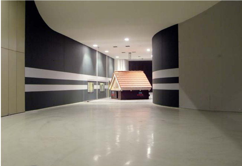
Picture 8: Wind tunnel with test house in the high-speed area
