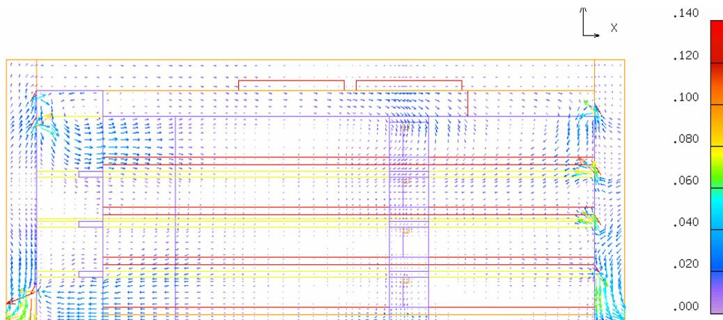
Figure 5 Vectors of air flow, opened facades, East-West direction
